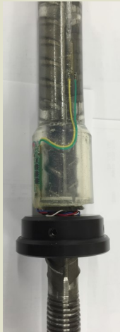
Strain sensor with rear centralizer installed on bolt
