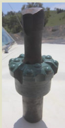
Ø100 mm reamer bit to increase diameter of bolt hole at collar
