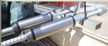
Sensors with protection tubes ready for installation
